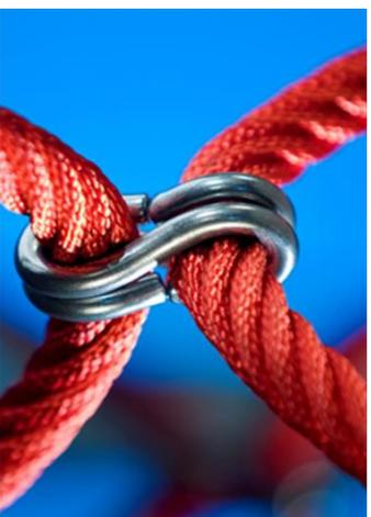
Corocord 'S'-clamps are used as universal connections in Corocord products. 8mm stainless steel rods with rounded edges are pressed around the ropes with a special hydraulic press, making them the ideal connector: safe, durable and vandalism-proof, all while allowing the typical movement of rope play structures.
