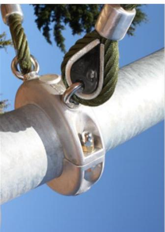
Corocord aluminium clamps are used as connectors between steel posts and rope. Two aluminium castings are bolted together. The height of the clamps is thus variable.
